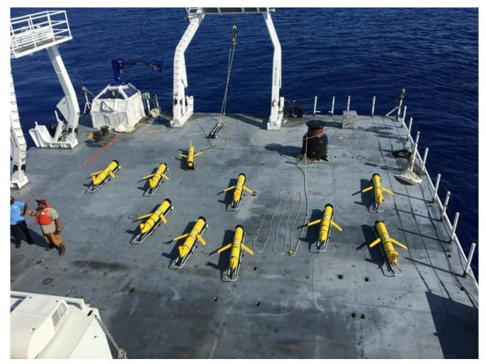
Naval Oceanographic Office personnel prepare to launch 10 littoral battlespace sensing gliders from USNS Maury in the Eastern Atlantic Ocean in support of NAVOCEANO's goal to deploy more than 50 gliders globally. These gliders are unmanned underwater vehicles used to collect data that is incorporated into ocean models, ultimately providing underwater forecasts for U.S. Navy operations. NAVAL OCEANOGRAPHY / Rebecca Shaw Unmanned Expertise
