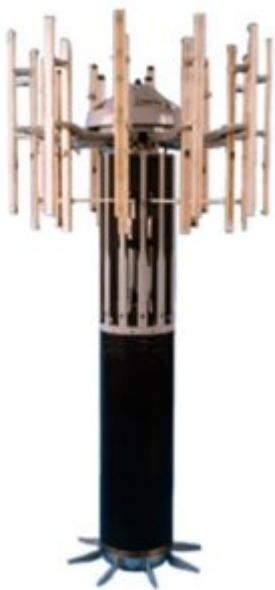
ALFS Airborne dipping sonar onboard MH-60R helicopter © Lockheed Martin.
