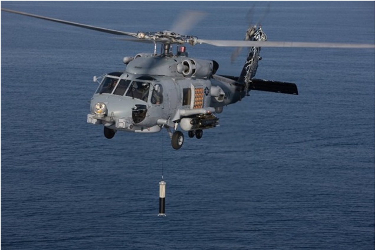
ALFS Airborne dipping sonar onboard MH-60R helicopter © Lockheed Martin.
