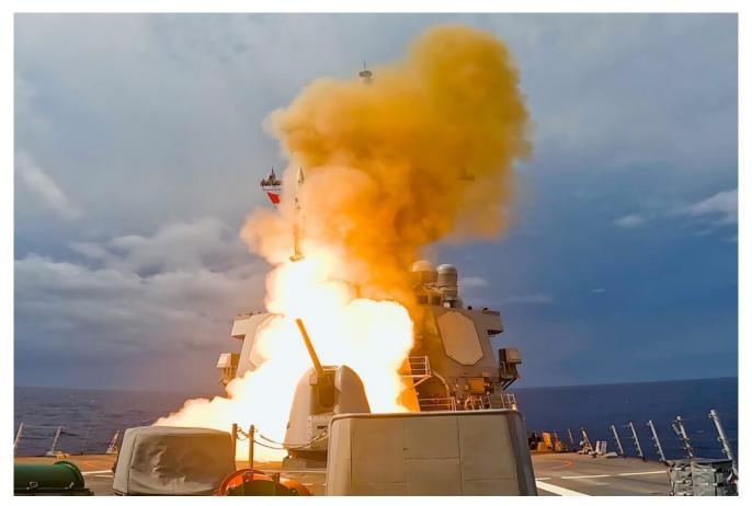
The Arleigh Burke-class guided-missile destroyer USS Higgins (DDG 76) launches a Raytheon-built Standard Missile (SM) 2 from a forward launcher while operating in the Philippine Sea, April 5. *U.S. Navy* | *MC1 Hannah Fry*
