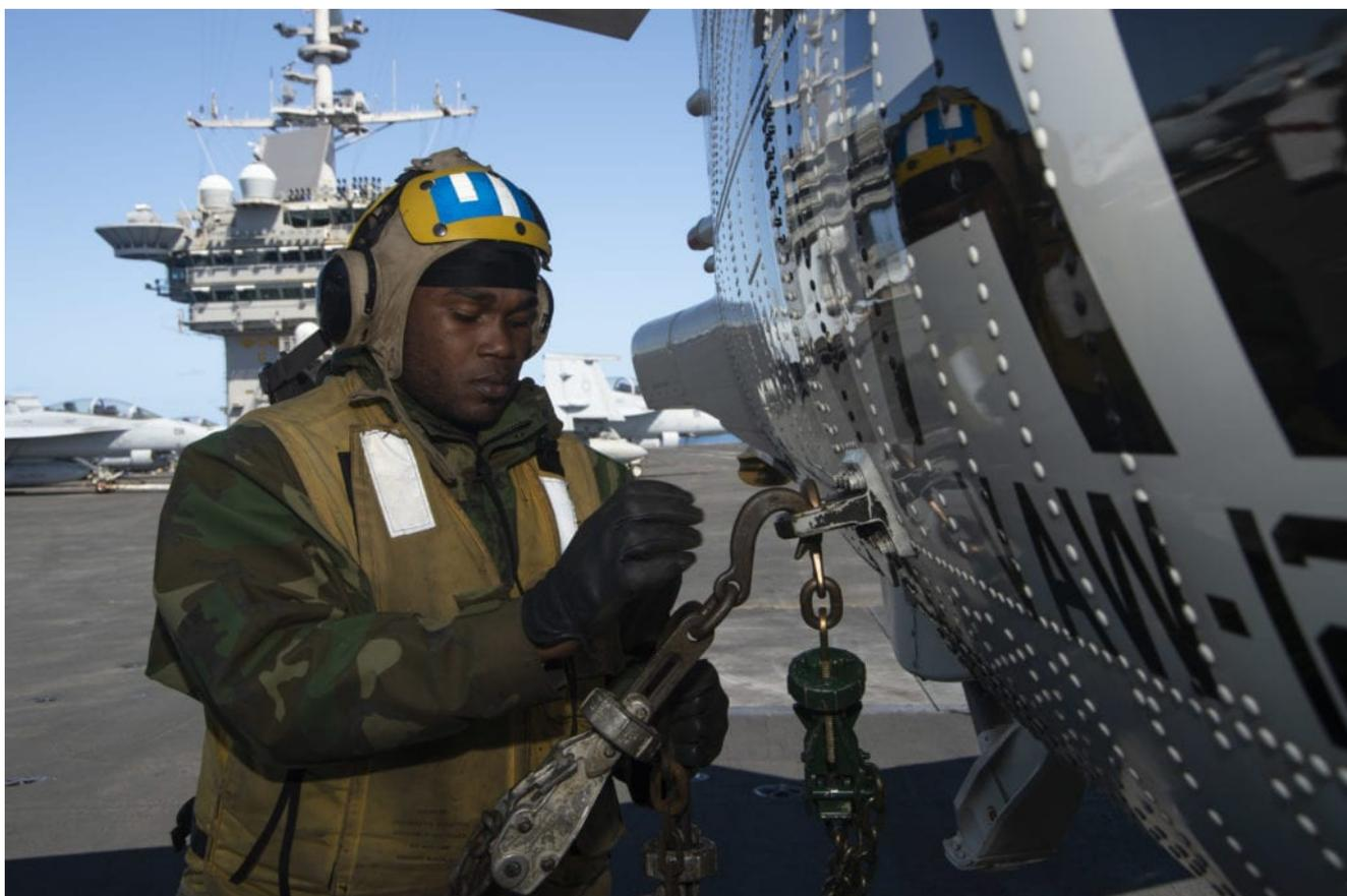
Aviation Boatswain's Mate (Handling) 2nd Class Albert Gibson chains an E-2D Hawkeye to the flight deck of the USS Harry S. Truman in the Atlantic Ocean on April 11. The Truman Carrier Strike Group is conducting operations there. U.S. Navy/Mass Communication Specialist Seaman Bela Chambers
