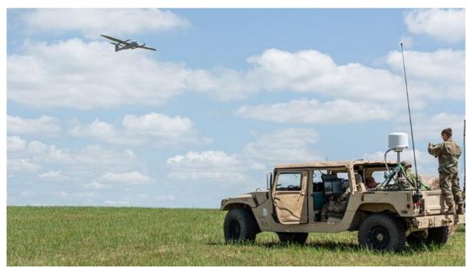
JUMP 20 is a VTOL, fixed-wing unmanned aircraft system that can be deployed quickly and requires no launch equipment or runway. *AEROVIRONMENT*
