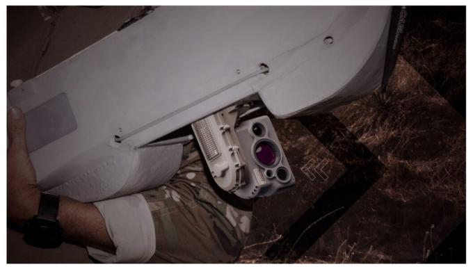
AeroVironment's new Mantis i45N imaging payload, intended for nighttime imaging. *AEROVIRONMENT*
