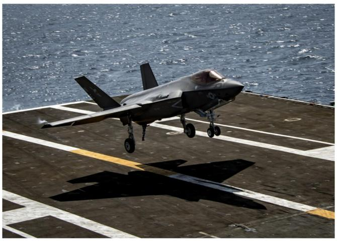
An F-35C from Strike Fighter Squadron (VFA) 147 lands on the flight deck of USS Carl Vinson (CVN 70) during flight deck and carrier air traffic control center certification. JPALS initial operational capability was declared following the successful installation, integration and flight certification of the first JPALS production unit aboard USS Carl Vinson in December 2020. JPALS is currently being deployed on all U.S. Navy aircraft carriers and amphibious assault ships. Japan
