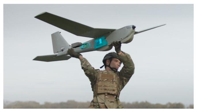
An illustration of a Puma small UAS equipped with the new Puma VNS, which determines the precise location of an aircraft during flight without relying on GPS. *AEROVIRONMENT*
