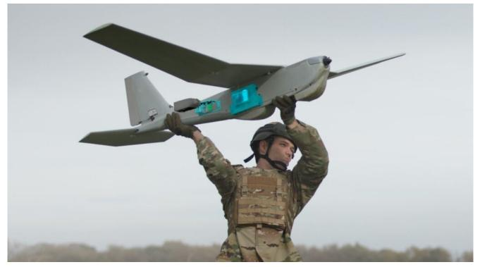
An illustration of a Puma small UAS equipped with the new Puma VNS, which determines the precise location of an aircraft during flight without relying on GPS. *AEROVIRONMENT* ARLINGTON, Va. – AeroVironment Inc. on Sept. 15 introduced
