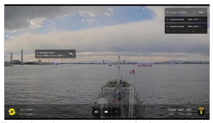
The AI-ris marine computer vision navigation sensor's view. SEA MACHINE ROBOTICS
