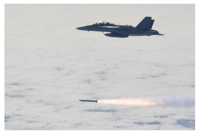
An AARGM-ER is successfully launched from a U.S. Navy F/A-18 Super Hornet during a recent test at the Point Mugu Sea Range, California. U.S. NAVY LOS ANGELES — Northrop Grumman Corp. announced Feb. 7 the successful completion of the second flight test of its AGM-88G Advanced Anti-Radiation Guided Missile Extended Range.
