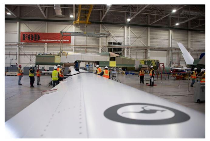
Australia's first MQ-4C Triton fuselage is lowered onto the unique one-piece wing.  $NORTHROP\ GRUMMAN$
