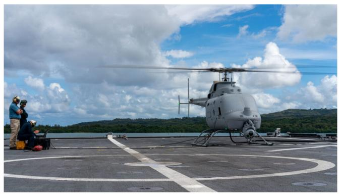
Sailors attached to Helicopter Sea Combat Squadron (HSC) 23, assigned to the Independence-variant littoral combat ship USS Jackson (LCS 6) and Naval Engineering Technology (NET) technicians perform ground turns on an MQ-8C Fire Scout on the flight deck of Jackson. U.S. NAVY / Mass Communication Specialist 3rd Class Andrew Langholf ARLINGTON, Va. – The newest version of the Navy's Fire Scout UAV is being prepared for deployment to the Western Pacific, according to an official photograph.
