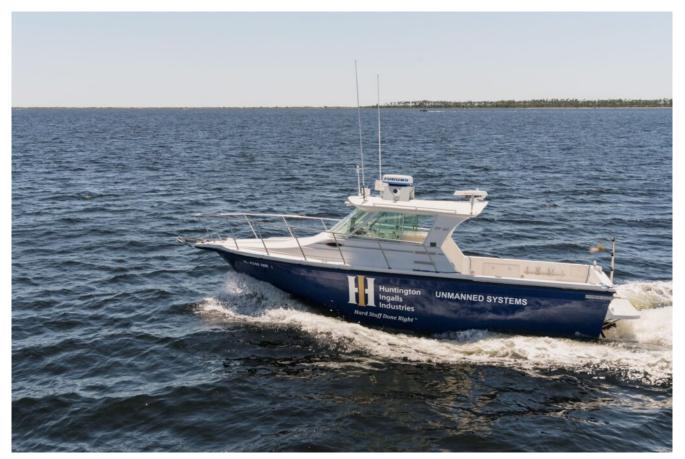
The Proteus unmanned surface vessel, outfitted with Sea Machines Robotics' SM300 autonomy system. *HUNTINGTON INGALLS INDUSTRIES*
