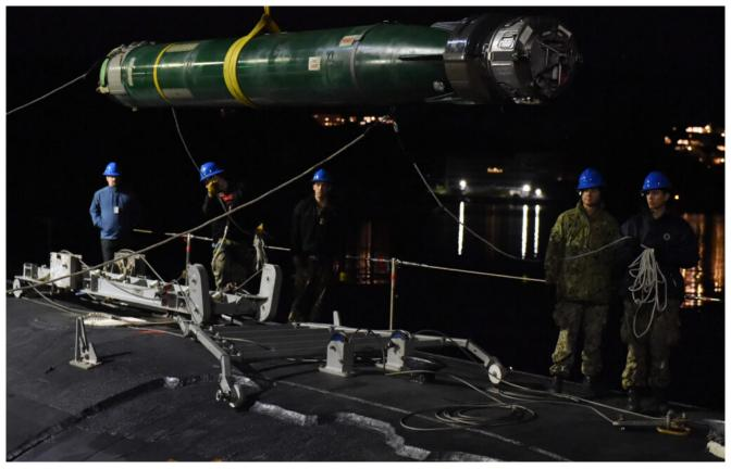
Sailors assigned to the Virginia-class, nuclear-powered, fast-attack submarine USS Minnesota (SSN 783) guide an MK-48 Advanced Capability torpedo during an expeditionary ordnance onload at the Haakonsvern Naval Base in Bergen, Norway, Oct. 18, 2019. U.S. NAVY / Chief Mass Communication Specialist Travis Simmons
