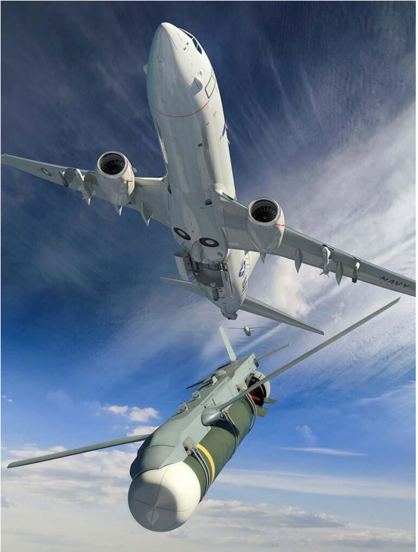
In an artist's rendering, a High Altitude Anti-Submarine Warfare Weapon Capability, or HAAWC, deploys from a Boeing P-8A Poseidon multi-mission maritime patrol aircraft. Boeing illustration
