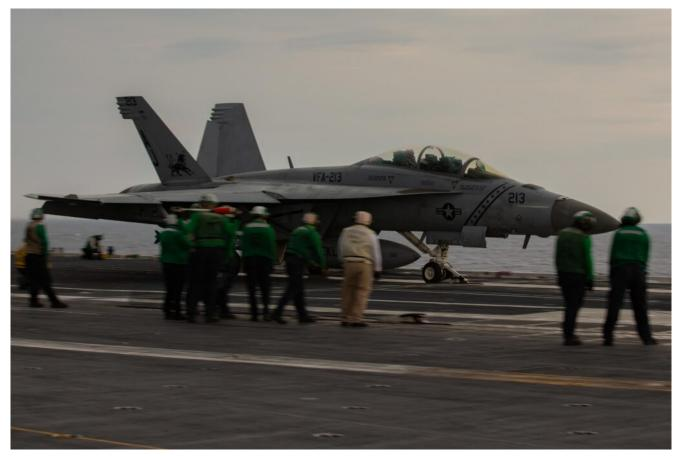
An F/A-18F Super Hornet from Strike Fighter Squadron (VFA) 213 launches off of the flight deck of the first-in-class aircraft carrier USS Gerald R. Ford (CVN 78) using the Electromagnetic Aircraft Launching System (EMALS), March 10, 2023. As the first-in-class ship of Ford-class aircraft carriers, CVN 78 represents a generational leap in the U.S. Navy's capacity to project power on a global scale.
