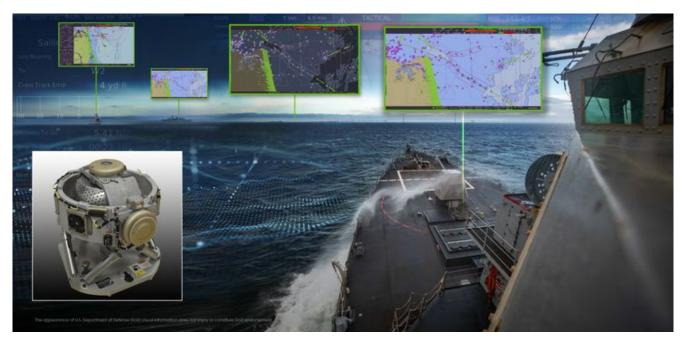
The Northrop Grumman-built AN/WSN-12 Inertial Sensor Module provides accurate positioning data with or without GPS for Navy ships and submarines. (Photo Credit: U.S. Navy)
