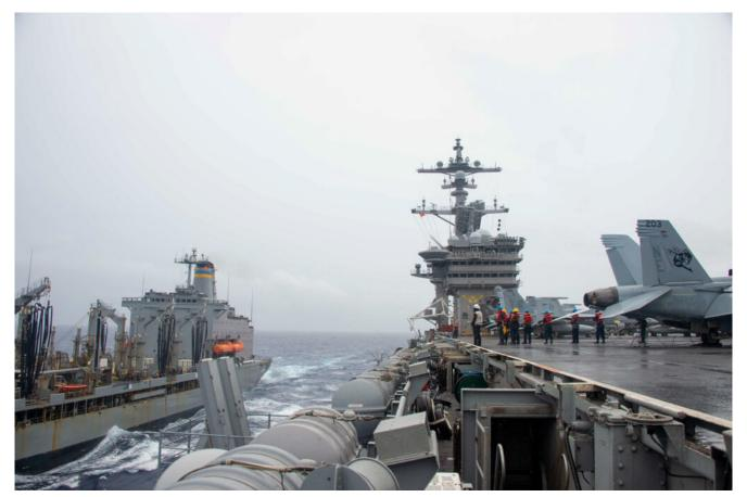
Nimitz-class aircraft carrier USS Carl Vinson (CVN 70) conducts a replenishment-at-sea with Henry J. Kaiser-class fleet replenishment oiler USNS Rappahannock (T-AO 204), The next-generation logistics ship is intended to be a smaller than current combat logistics force ships such as the Rappahannock. U.S. NAVY / Mass Communication Specialist Seaman Elizabeth Grubbs
