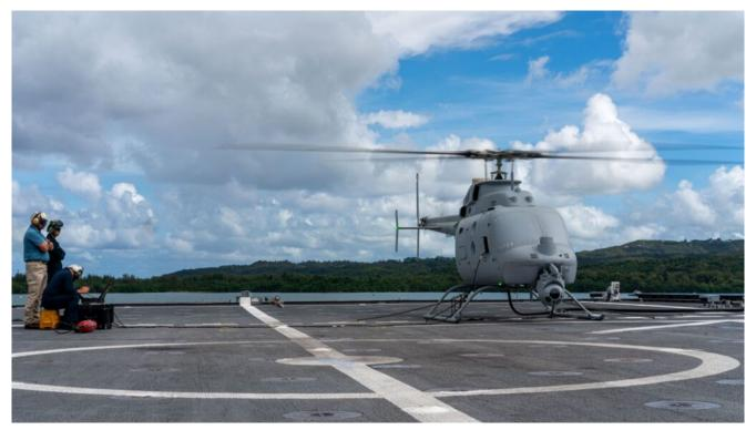
Sailors attached to Helicopter Sea Combat Squadron (HSC) 23, assigned to the Independence-variant littoral combat ship USS Jackson (LCS 6) and Naval Engineering Technology (NET) technicians perform ground turns on an MQ-8C Fire Scout on the flight deck of Jackson. U.S. NAVY / Mass Communication Specialist 3rd Class Andrew Langholf
