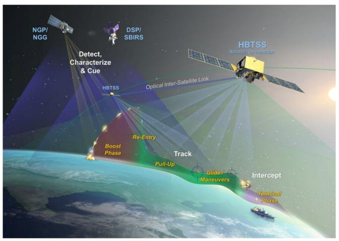
A graphic illustrates how Hypersonic and Ballistic Tracking Space Sensor satellites would provide continuous tracking and handoff to enable targeting of enemy missiles launched from land, sea or air. NORTHROP GRUMMAN
