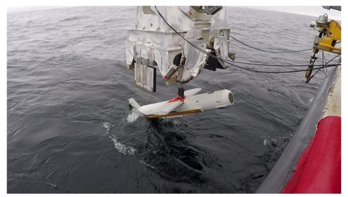
The AN/AQS-20C Towed Mine-hunting Sonar is streamed into Gulf of Mexico waters of the Naval Surface Warfare Center Panama City Division (NSWC PCD) Gulf test range. Developmental Testing was completed on Feb. 12, 2019. The testing marks completion of incorporating the 'Charlie' variant sonar sensor modernization. U.S. NAVY / Eddie Green
