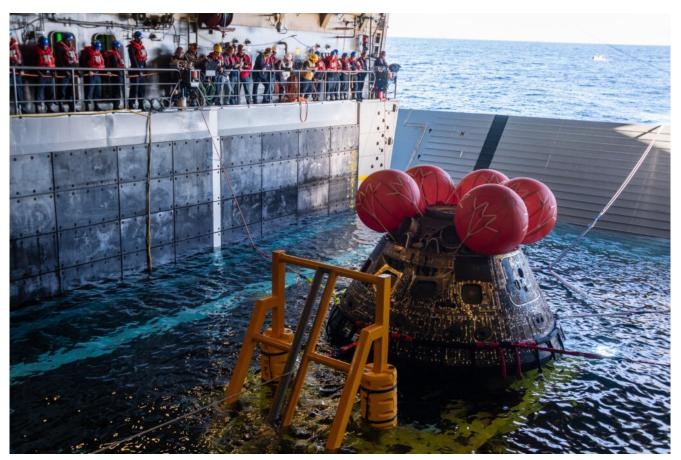
Sailors aboard the amphibious transport dock USS Portland (LPD 27) use a line load attenuating mechanism assembly to pull the NASA Artemis I Orion spacecraft into the well deck, Dec. 11, 2022. U.S. NAVY/ Mass Communication Specialist 2nd Class Devin Kates
