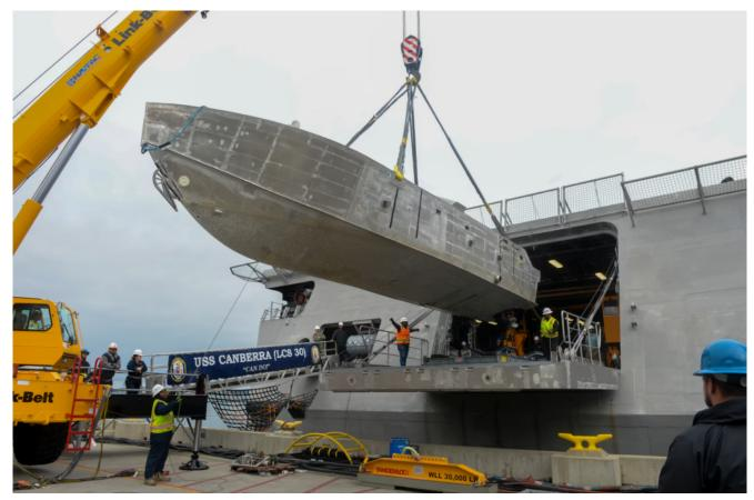
A mine countermeasures unmanned surface vehicle is craned aboard the Independence-variant littoral combat ship USS Canberra (LCS 30), as a part of the first embarkation of the Mine Countermeasures (MCM) mission package, April 23. (U.S. Navy photo by MC1 Vance Hand)
