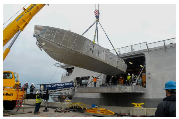
A mine countermeasures unmanned surface vehicle is craned aboard the Independence-variant littoral combat ship USS
