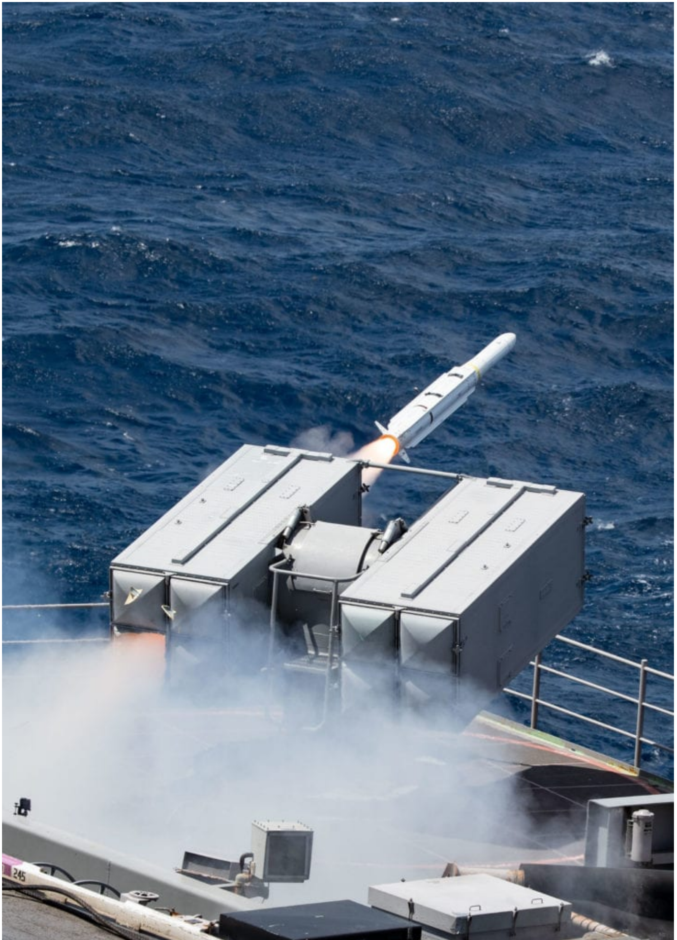
An evolved sea sparrow missile (ESSM) launches from one of USS Gerald R. Ford's (CVN 78) weapons sponsons during combat
