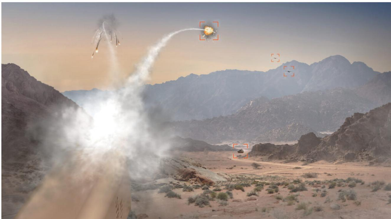
70mm rockets guided by APKWS guidance kits went 5 for 5 against agile, high-speed Class-2 unmanned aerial systems in testing. *BAE SYSTEMS*
