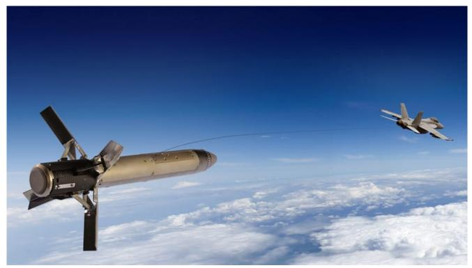
An artist's rendering of a BAE Systems ALE-55 Fiber-optic towed decoy deployed on an F/A-18 Super Hornet strike fighter. BAE Systems
