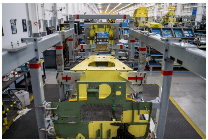
The cabin of an Czech Republic AH-1Z is loaded onto the manufacturing line at the Amarillo Assembly Center to begin production. *BELL TEXTRON*
