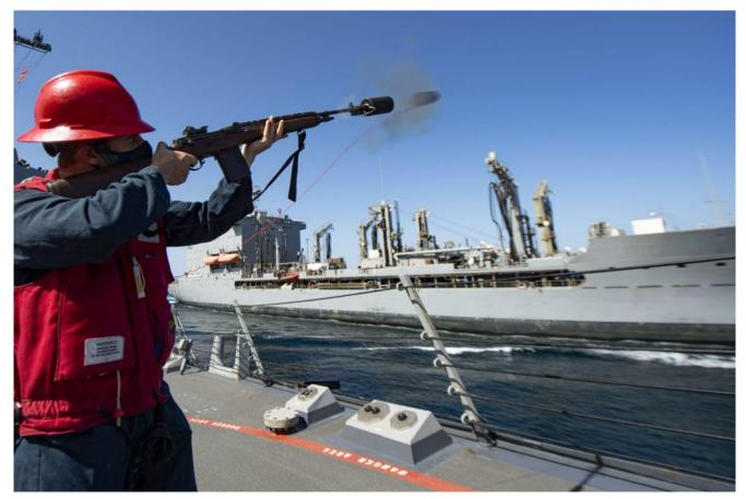
Gunner's Mate 3rd Class Gage Duncan, from Cardington, Ohio, fires a shot line from the deck of the guided-missile destroyer USS Sterett (DDG 104) to the fleet replenishment oiler USNS Leroy Grumman (T-AO 195) during a replenishment-at-sea. U.S. Navy / Mass Communication Specialist Seaman Drace Wilson
