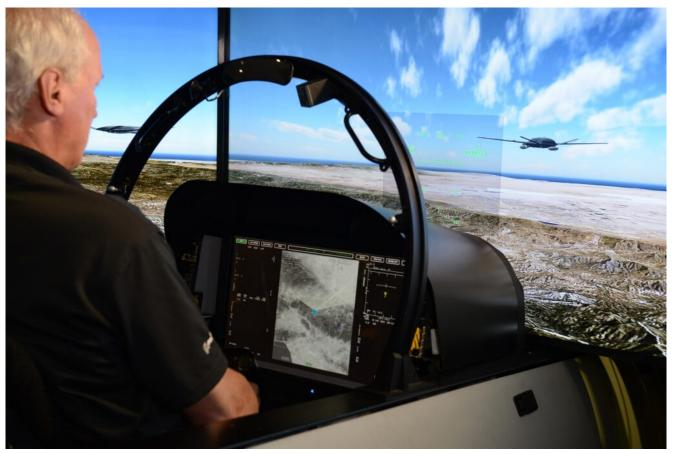
Boeing's MUM-T demonstration included three different naval aircraft tasking four virtual, autonomous MQ-25s to conduct intelligence, surveillance and reconnaissance missions. Here a simulated F/A-18 Super Hornet interacts with a simulated MQ-25. *BOEING*
