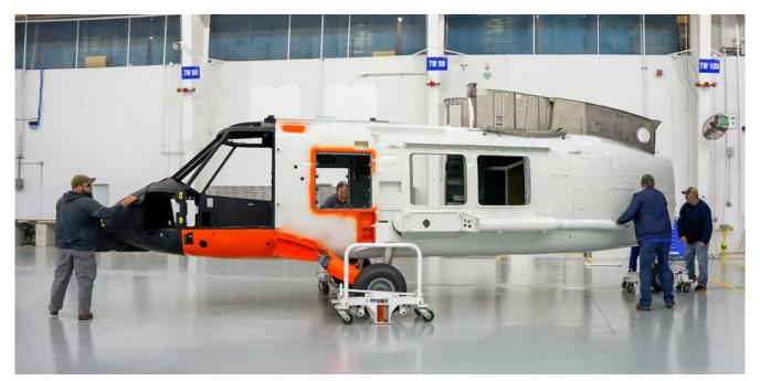
Sikorsky delivered the first of 45 new airframes to the Coast Guard for the service-life extension of the service's MH-60T helicopter fleet. \*\*\*\*\*
