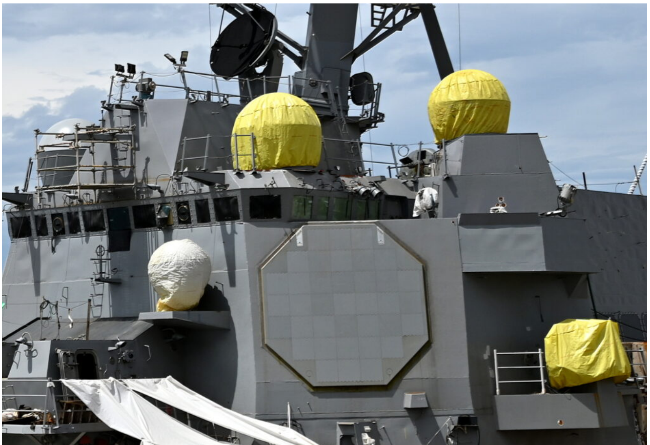
The fixed-face antenna of the SPY-6-(V)1 radar is shown on the
