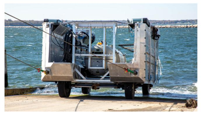
HII collaborated with the U.S. Navy on a research and development effort that advanced the launch and recovery of a large size unmanned undersea vehicle, using an amphibious ship and HII's Pharos system. *HII*
