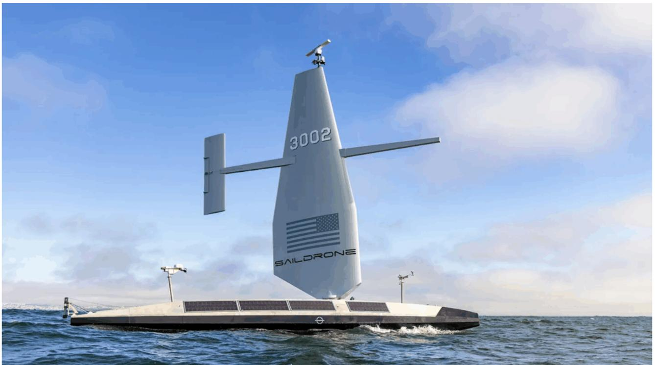
The Saildrone Surveyor is a 20-meter USV capable of long-endurance missions in the open ocean, collecting deep-ocean bathymetry and performing a wide range of maritime domain awareness tasks—from anti-submarine warfare (ASW) to trans-ocean cable route surveys.
