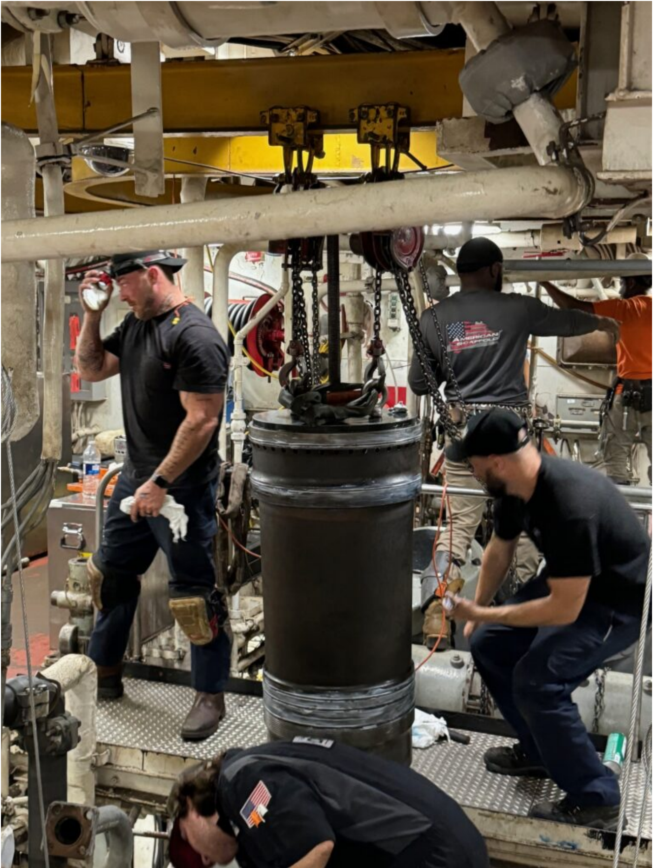
Fairbanks Morse Defense workers overhaul an engine using the "pit stop" method. Photo credit: Fairbanks Morse Defense Imagine if a Navy ship could pull into a pit stop like a race car, get its engine overhauled and be back on the seas in less
