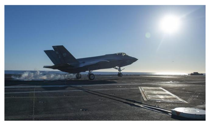
An F-35C Lightning II, from the "Rough Raiders" of Strike Fighter Squadron (VFA) 125, makes an arrseted gear landing on the flight deck of the aircraft carrier USS Nimitz. Joint Precision Approach and Landing Systems (JPALS) has been supporting F-35B deployments on U.S. Navy LH-class amphibious assault ships since 2016 and F-35C deployments on U.S. Navy aircraft carriers since 2021.
