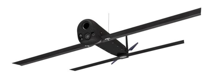
AeroVironment's Switchblade 300 loitering munition, which can now be integrated with the larger JUMP 20 unmanned aircraft. *AEROVIRONMENT*
