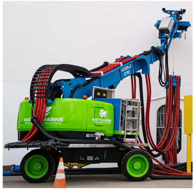
The "world's first" port with three ship shore power systems for cruise liners to turn off diesel engines and connect to shoreside electricity to reduce emissions
