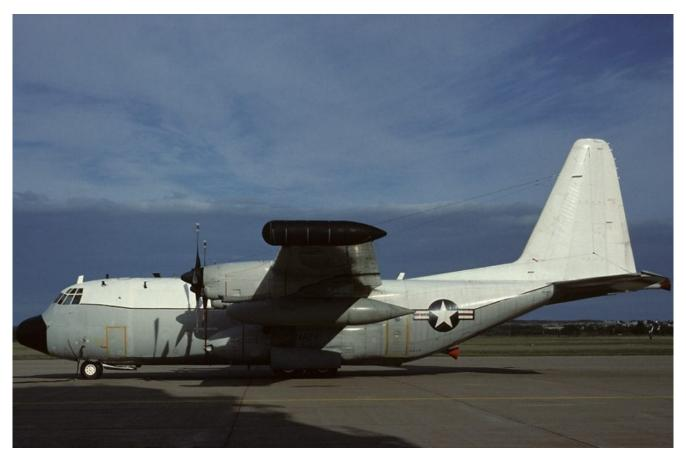
A Lockheed EC-130Q Hercules, which previously handled the Navy's TACAMO work. The Navy has now decided to acquire the C-130J-30 Super Hercules as its platform for communicating with deployed ballistic-missile submarines. WIKIPEDIA / Alain Rioux
