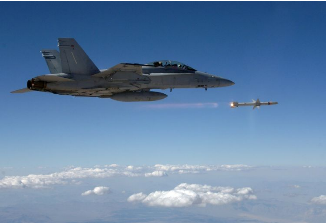
An AGM-88E2 AARGM is launched from an F/A-18 during testing. NORTHROP GRUMMAN
