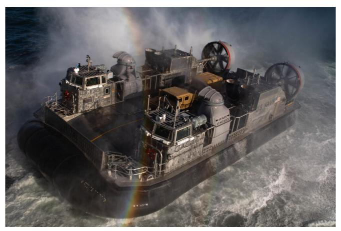
Landing Craft, Air Cushion (LCAC) 104, attached to Assault Craft Unit 4, approaches the Wasp-class amphibious assault ship USS Kearsarge (LHD 3) for well deck operations Dec. 1, 2022. LCAC 100 is the Navy and Marine Corps next generation landing craft designated to replace the legacy LCAC, providing a more reliable and capable high speed amphibious connector to deliver Sailors and Marines and their equipment from ship to shore. U.S. NAVY / Mass Communication Specialist Mark O. Klimenko
