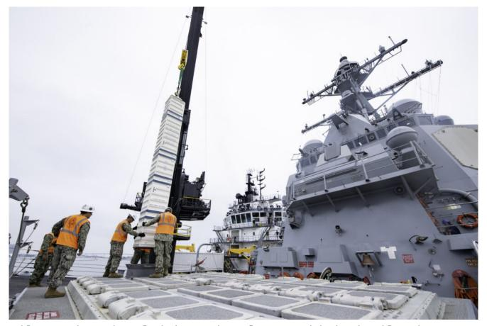
Sailors aboard Arleigh Burke-class guided-missile destroyer USS Spruance (DDG 111) guide training ordnance into the ship's forward vertical launch system (VLS) cells during a proof-of-concept evolution in San Diego, Oct. 4. U.S. NAVY / Mass Communication Specialist 3rd Class Taylor Crenshaw
