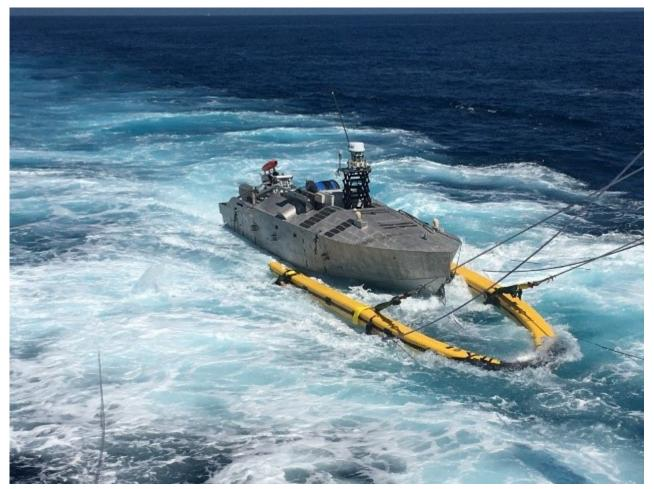
The Minecountermeasure Unmanned Surface Vehicle is recovered onboard USS Manchester (LCS 14) during Unmanned Influence Sweep System initial operational test and evaluation June 2021. U.S. NAVY
