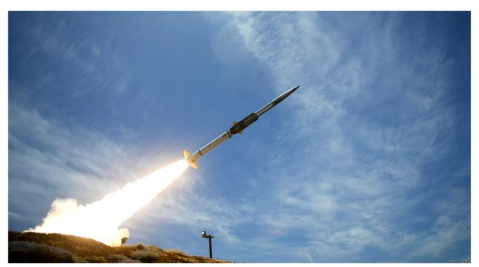
Northrop Grumman's GQM 163-A Coyote, a target vehicle used to simulate advanced anti-ship cruise missile threats. NORTHROP GRUMMAN
