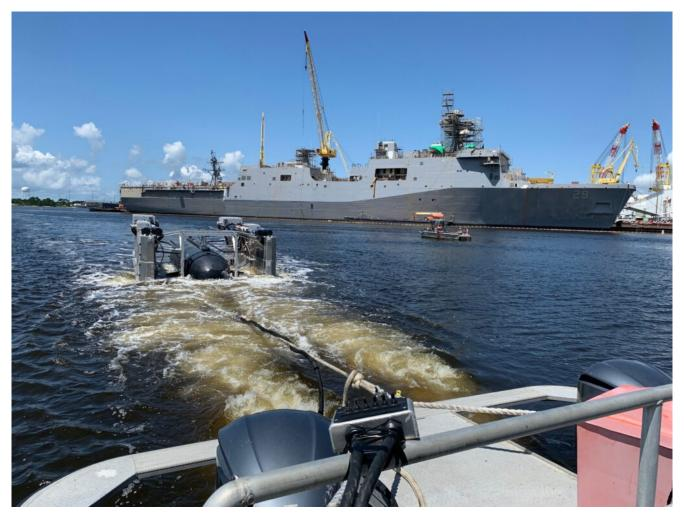
HII's prototype Pharos platform being towed behind a vehicle in the Pascagoula River while recovering HII's LDUUV during a June 8 demonstration. HII
