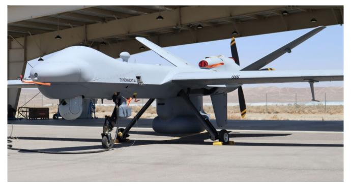
An MQ-9A Block 5 remotely piloted aircraft equipped with a Leonardo Seaspray 7500E V2 multi-mode radar. *GENERAL ATOMICS AERONAUTICAL SYSTEMS*
