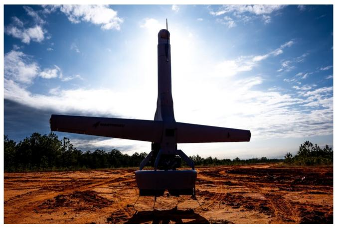
A V-BAT vertical takeoff and landing unmanned vehicle. MARTIN UAV
