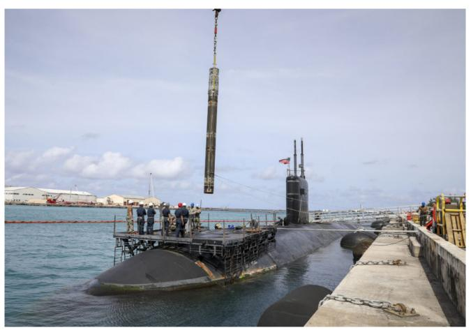
A Tomahawk cruise missile is removed from Los Angeles-class attack submarine USS Asheville at Polaris Point, Guam. An SLCM-N would occupy the place in naval armament formerly occupied by the now retired nuclear-armed version of the Tomahawk. U.S. NAVY / Mass Communication Specialist 1st Class Victoria Kinney
