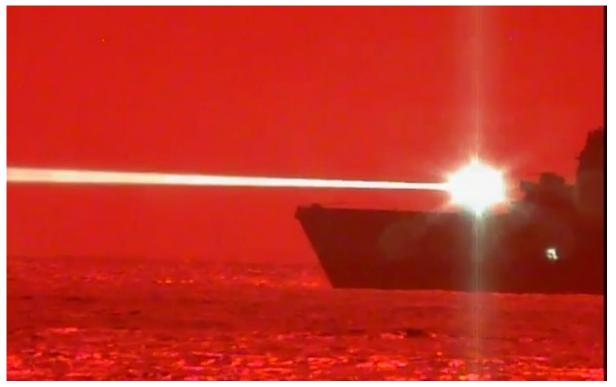
1001 Amphibious transport dock ship USS Portland (LPD 27) successfully disabled an unmanned aerial vehicle with a solidstate laser, Technology Maturation Laser Weapon System Demonstrator (LWSD) MK 2 MOD 0 in May 2020 in this still image from U.S. Navy video from Pacific Fleet Public Affairs. U.S. NAVY
