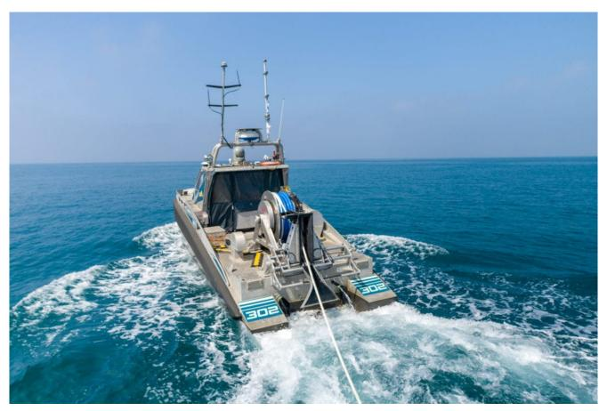
Elbit Systems has integrated the TRAPS-USV with its Seagull unmanned surface vehicle. Elbit Systems
