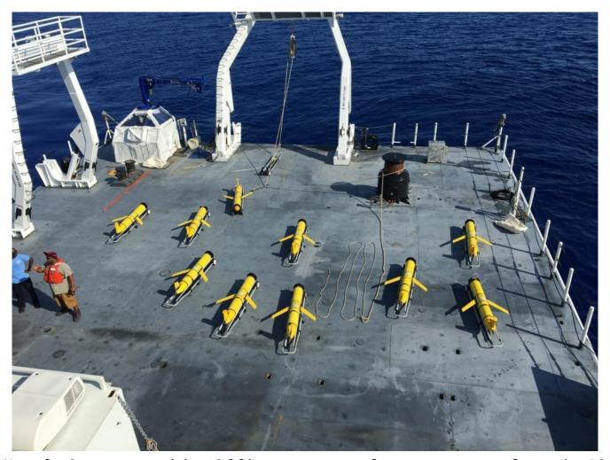
Naval Oceanographic Office personnel prepare to launch 10 littoral battlespace sensing gliders from USNS Maury in the Eastern Atlantic Ocean in support of NAVOCEANO's goal to deploy more than 50 gliders globally. These gliders are unmanned underwater vehicles used to collect data that is incorporated into ocean models, ultimately providing underwater forecasts for U.S. Navy operations. NAVAL OCEANOGRAPHY / Rebecca Shaw
